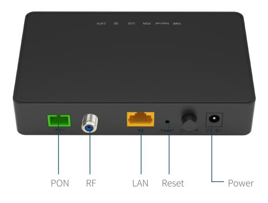
• Interfaces: 1 x SC/APC GPON Port, 1 x 10/100/1000Mbps LAN Port, 1 RF Port • Buttons: Power ON/OFF Button, Reset Button • Power Supply: DC 12V 0.5A
